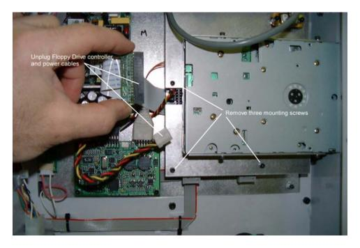
Next, swing the floppy up from the bottom. To do this, you will have to move it left slightly to get it out of the access door hole. (Be care of the CPU power plug in the notch behind the floppy)
